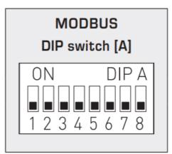
The device address in the range of 1 to 247 is set at DIP switch [A].
