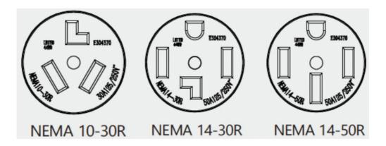
If you're using a standard dryer plug, choose the CGB J1 or J2 model that corresponds to your plug type (NEMA 10-30 or 14-30). If your electrician has installed a 50amp service, choose the CBG J3 model (NEMA 14-50).
