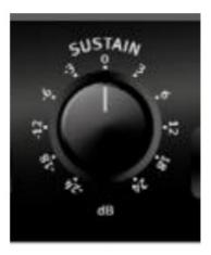
Sustain can be used to increase or attenuate the sustain phase of a signal by up to 24 dB. Positive sustain values extend the sustain.
