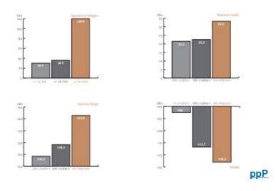
When it comes to volume, the 120-volt technology exhibits a performance that is twice that of common components and circuits, in regard to maximum level and dynamic range, with values that are approximately 10 dB higher. THD measurements of the SPL op-amps show a difference of more than 3 dB compared to the OPA134 at 36 V — in terms of sound pressure level, that corresponds to an improvement of more than 50%. The operating level most commonly used for audio equipment is 30 volts
