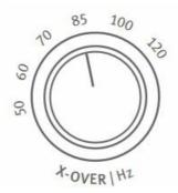
Select the X-OVER frequency (50, 60, 70, 85, 100 or 120 Hz) with the MID-HI X-OVER switch (4).
