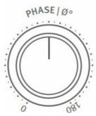
• If you set the Phase switch to position "Var 0°", you set the phase of the LOW signal with the phase potentiometer from 0° to 180°.
