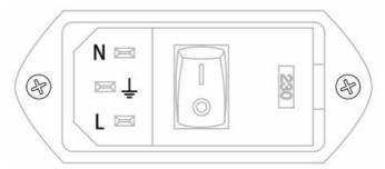
Mains voltage (switchable): 230 V AC / 50 Hz or 115 V AC / 60 Hz
