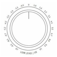
Set the overall level of the subwoofer(s) with the LOW LEVEL potentiometer (10). The control has a range of +/-10dB. It allows to finely control the level of your subwoofer(s) in relation to your top speakers.
