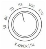
The LOW crossover filter is a Linkwitz/Riley design. The roll-off is 24 dB per octave. Set the crossover frequency with the LOW X-OVER switch (3). Available crossover frequencies are: 50, 60, 70, 85, 100 and 120 Hz.
