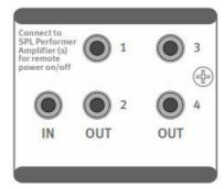
If you own an SPL device supporting AMP CTL output(s) you can trigger standby and operation of the Crossover. Therefore connect the AMP CTL output of the SPL device to the Crossover's AMP CTL IN (19).
