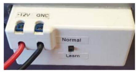
2. The switch at the back is set to "Normal" during standard operation.
