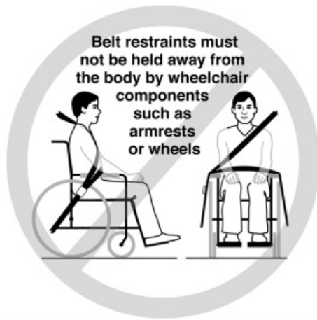
Figure 3a - Improper positioning of pelvic-belt restraints over wheelchair supports.
