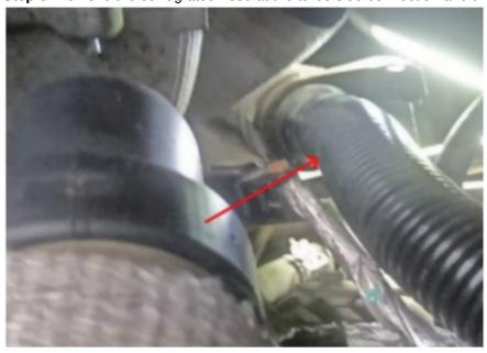
**Step 9**: Install the rubber boot and clamp.(This clamp is not included in the package.)
