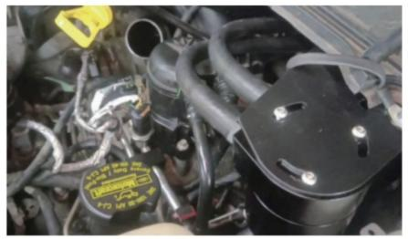
**Step 26**: Reinstall the hot-side intercooler pipe. (1x worm gear clamps, 1x spring clip) Congratulations! You have finished installing the 2011-2016 Ford 6.7L Powerstroke CCV Reroute/Delete w/Catch Can Internal External Kit
