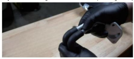
**Step 12**: Grease the O-ring groove on the aluminum adapter and place the thin o-ring within the groove.
