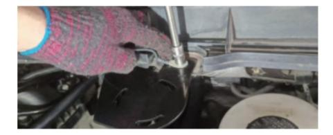
**Step 21**: Thread the fittings onto the catch can. Tighten the fittings with a wrench.
