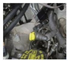
Step 15: Install the CCV adapter and aluminum plug.
