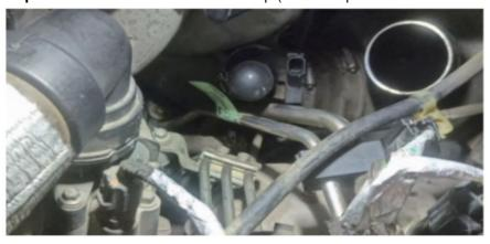
**Step 10**: Attach the shorter hose to the top barb (1x worm grar clamp) **Step 11**: vAttach the longer hose to the bottom barb (1x worm grar clamp)
