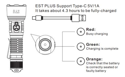
\*Note: Only can charge rechargeable 18650 lithium battery. EST PLUS can not work when charging.
