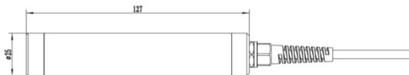
Figure 2 External dimension of the dissolved oxygen sensor
