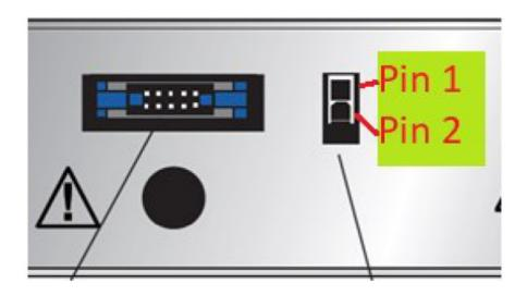
Please see Molex connector product page for range of mating receptacles (for example, Molex receptacle part number: 39012020, crimps part number: 39000038, and wire gauge of 18 to 24 AWG): <a href="https://www.molex.com/molex/products/part-detail/pcb\_headers/0039301022">https://www.molex.com/molex/products/part-detail/pcb\_headers/0039301022</a>
