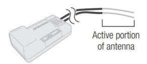
NOTICE: Do not cut, kink, or modify the antennas. Damage to the coaxial portion of an antenna will reduce the
