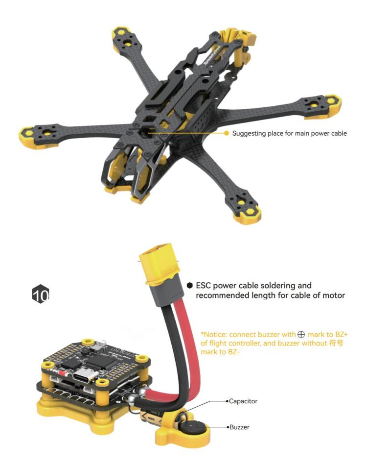
Inner motor wire recommended length: 110mm
