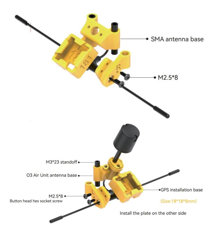
(\*Note: pictures for assembly reference only. Frame doesn't include antenna)
