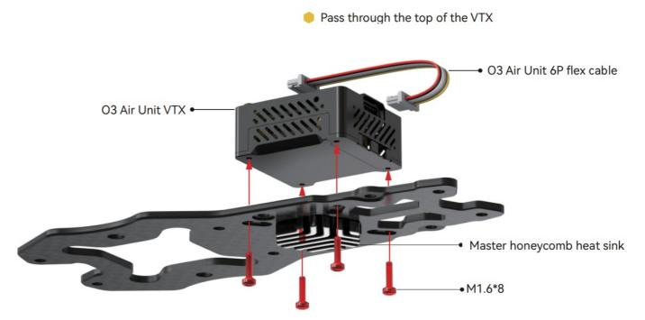
The 4 original screws at the bottom of the O3 Air Unit need to be removed
