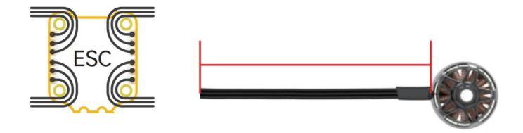
Outer motor wire recommended length: 93mm
