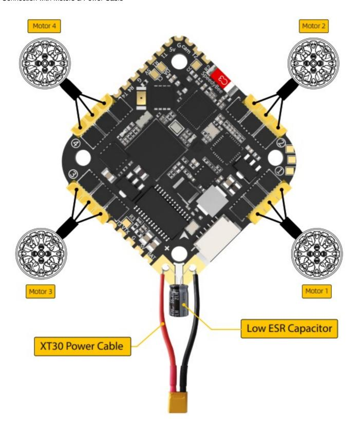
**Note:** In order to prevent the AIO from being burnt out instantaneous voltage spikes on powering up, it is strongly recommended to use the Low ESR capacitor in the package.
