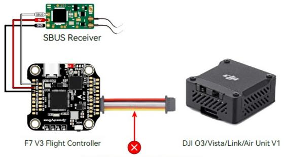
Do NOT connect this wire to assure the external SBUS receiver work properly!
