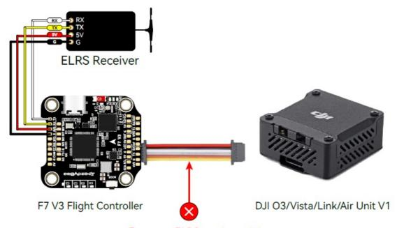
For some ELRS receivers, it is necessary to disconnect this wire in order to function properly!
