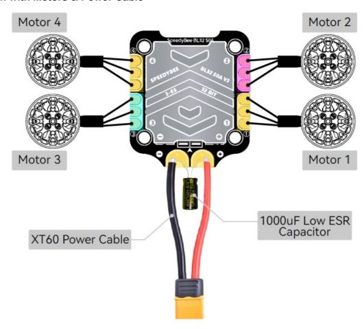
**Note**: In order to prevent the stack from being burnt out instantaneous voltage spikes on powering up, it is strongly recommended to use the Low ESR capacitor in the package.
