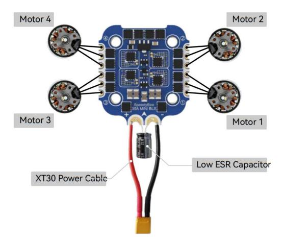
■ Note: In order to prevent the stack from being burnt out instantaneous voltage spikes on powering up, it is strongly recommended to use the Low ESR capacitor in the package.
