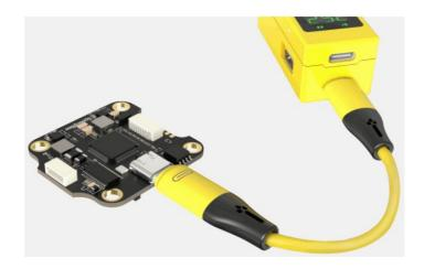
**NOTE 1** – It's safe to power Adapter 3 even if the data cable is connected to the main body on both ends.
