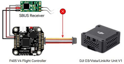
Do NOT connect this wire to assure the external SBUS receiver work properly
