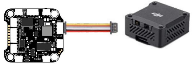
Use 6-pin cable comes with the F7 V3 stack (See the accessory No.3 in the package section)
