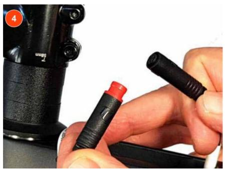
• Connect Ribelle connectors 1 and 2 to the connectors obtained in the previous steps. Be very careful to collimate the arrows during insertion!!
