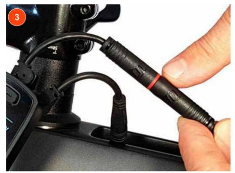
• Disconnect the connector with the middle red line.
