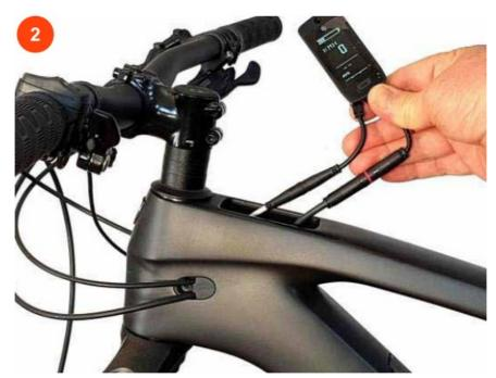
• Locate the connector with the middle red line.
