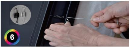
5. There are 2 different strength springs included. The black springs are the primary springs used on all 4 sides of the surface. The silver springs are extras and can be used to help resolve any tensioning issues that may arise. They are generally used in the corners (2 per corner) as needed. They can also be used to help add additional tension elsewhere on the surface as needed.
