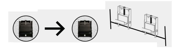
Fix the two mounting brackets along a level horizontal line.
