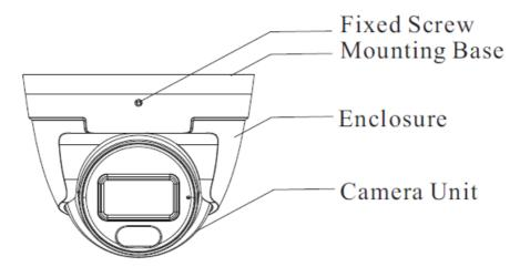
3. Route and connect the cables hen secure the mounting base to the ceiling or wall with the screws provided.
