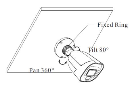
1. Drill the screw holeson the wall according to the drill template.
