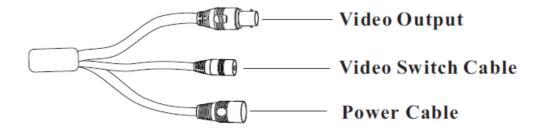
Video Switch: Four video output modes can be optional—AHD, TVI, CVI and CVBS (a) remove the cover of the video switch cable; (b) hold and press the button in the video switch cable for 5 seconds to switch the current video output.
