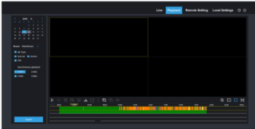
Click **Playback** to enter into Playback interface to remotely view the records in WIRELESS NVR HDD. It supports 1 to 4 channel record playback.
