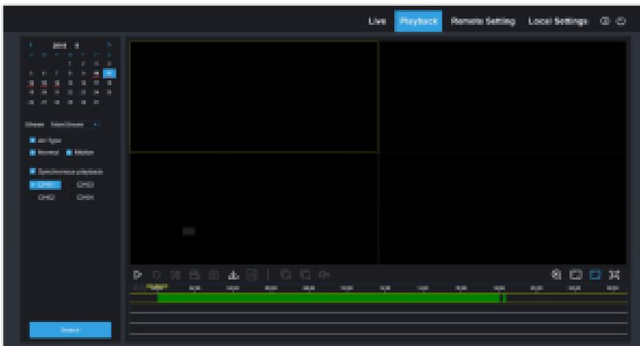
Second, select record type (Normal record, Motion record,PIR record) and channels, and then click **Search** and time axis panel will display specific time quantum. On the time axis, red part stands for motion record, green stands for normal record and original part stands for no record during this period.
