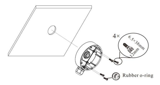
Fix the mounting base of the camera to the upper cover of the junction box.
