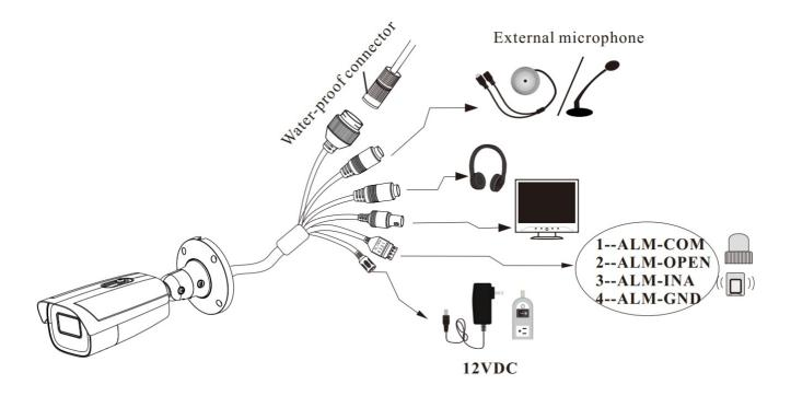
\* It is recommended to install the water-proof connector for outdoor installations.
