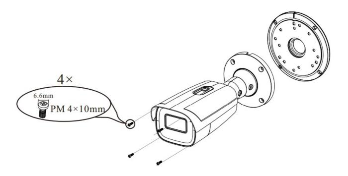
⑤ Route the cables through the cable hole and connect the camera. Then install the camera onto the mounting base of the junction box.
