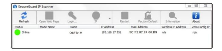
③ In the device list, you can view the IP address, model number, and MAC address of each device. Select the applicable device and double click to open up the web viewer. You can also manually enter the IP address in the address bar of the web browser.
