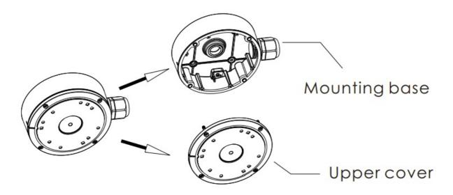
Attach the drill template of the junction box to the place where you want to install the junction box and thenrill the screw hole and calbe hole on the wall according to the drill template. Install junction box onto the wall by using the screws provided.
