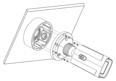
6. Bracket Adjustment-Loosen the fixed ring to adjust the view angle of the camera. After you get the optimum angle of view, tighten the fixed ring to complete the installation.
