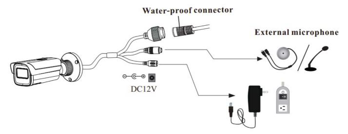
1 It is recommended to install the water-proof connector for outdoor installations.
