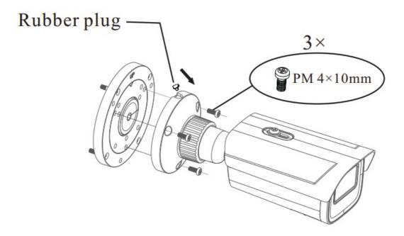
5. Connect the cables and then install the camera onto the junction
