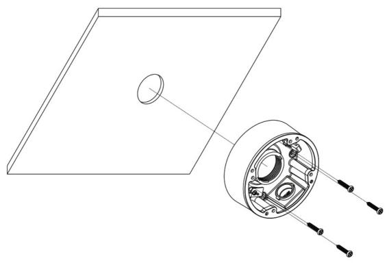
3. Mount the rubber plug to the gap of the mounting base and fasten the camera onto the mounting base.
