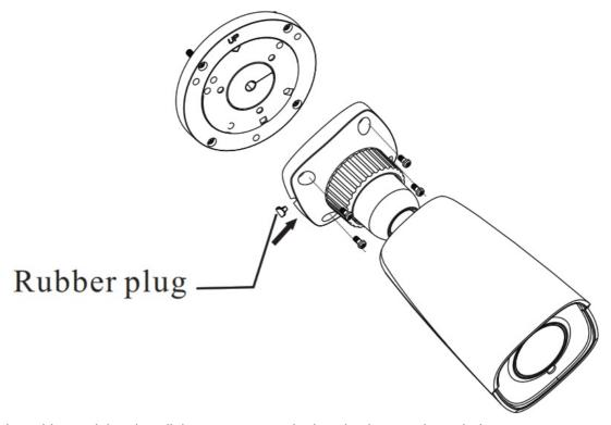
4. Connect the cables and then install the camera onto the junction box as shown below.
