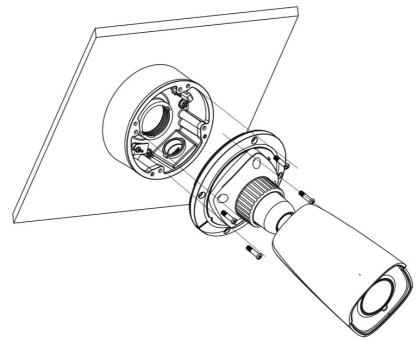
5. Bracket Adjustment-Loosen the fixed ring to adjust the view angle of the camera. After you get the optimum angle of view, tighten the fixed ring to complete the installation.
