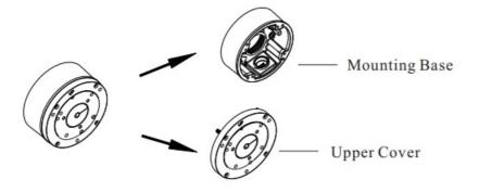
2. Install junction box onto the wall by using the screws provided.
