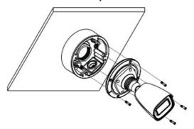
5. Bracket Adjustment-Loosen the fixed ring to adjust the view angle of the camera. After you get the optimum angle of view, tighten the fixed ring to complete the installation.
