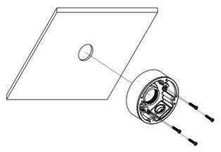
3. Fasten the camera onto the mounting base.
