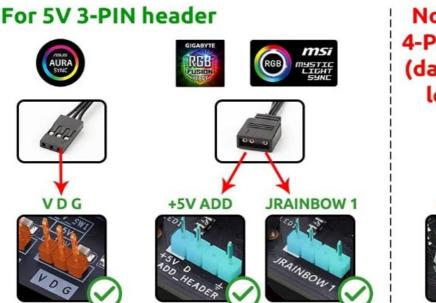
Not for 12V 4-PIN header (damage the led strip)
