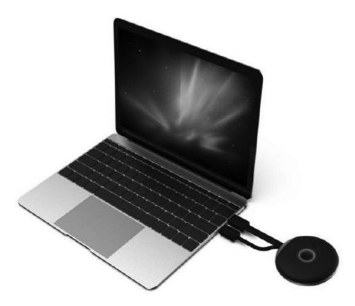
Set the transmitter with the control button up-wards next to your computer. The button should always be within range to start or stop the trans-mission.
