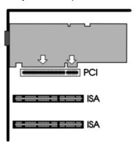
Installing the Card in a PCI Local Bus Slot
