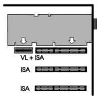
Installing the Card in a VESA Local Bus Slot
