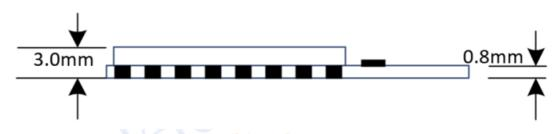
(b) Side View Fig. 3.1 Size for ESP-32S
