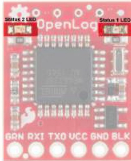
Status LEDs on the OpenLog.
