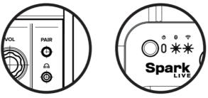
3. Press the Bluetooth Pair Button on the Rear Panel of Spark Control X and it will search for the nearest Spark amp as indicated by the flashing blue LED Connection Indicator on the Main Panel.
