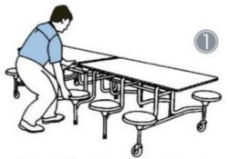
Release locking bar by pressing down on the table surface, with right hand lift clear the lock.
