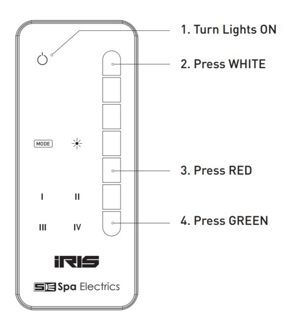
The iRIS lighting controller has a QUICK SETUP feature to program the MULTI PLUS lights for iRIS operation.
