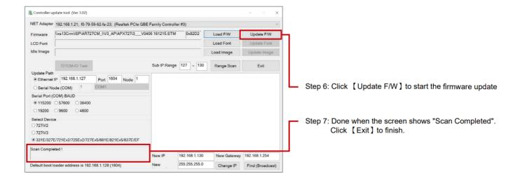
Way 2: Entering Boot Load Mode (When the 401-IO-0808R-U2 program does not work, you can use this method to re-download)
