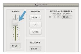
Pressing the arrow key fast will move the volume in 6db increments; signer presses will move the volume by 1db.
