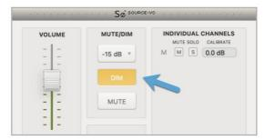
Pressing the Mute button will cut the volume output to minus infinity or the default ASCII key command of "shift+command+up arrow" is pressed the volume output will be reduced by minus infinity or the mute function will be disengaged if already engaged.
