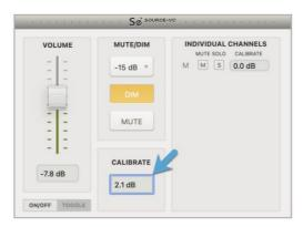
Under the "Individual channels" section, individual channels can be soloed by clicking on the "s" button or muted by pressing the "m" button by the assigned channel. The volume setting box can be used to calibrate by a fixed amount the specific channel so you can calibrate your monitor system.
