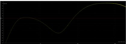
As displayed above, the FOCUS control significantly shapes the low-end response of the pedal.
