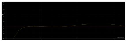
As you can see, there is not much of a tonal change when GRIT is enabled and all other controls are enabled, except for a minor treble fall-off beginning around 1100Hz.
