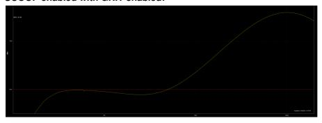
There is a mild interaction between GRIT and SCOOP which results in a smoothing out of the boosted treble frequencies with an earlier peak and a flatter curve. The severity of the treble boosting happening in the SCOOP circuit is reduced by just over 1dB when GRIT is enabled in this instance.
