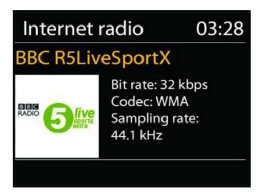
When you select Internet radio, ICD2020 directly contacts the Frontier Silicon Internet radio portal (which is supported by Airable) to get a list of stations.
