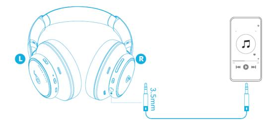
Play audio on an external device by plugging in a 3.5mm AUX cable. Wired listening will turn off Bluetooth mode automatically.
