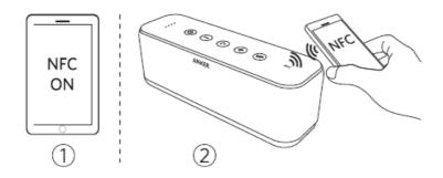
Note: To break connection, tap again the NFC device onto SoundCore's NFC detection area.
