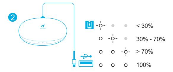
3. To check the battery level of the charging case, open it to activate the LED indicator.
