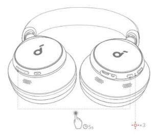
Press and hold the volume up and power button simultaneously for 5 seconds until the LED flashes red three times.
