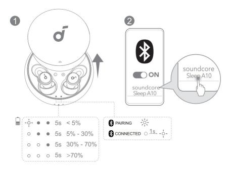
Open the charging case, the earbuds will automatically power on and enter pairing mode. Select "soundcore Sleep A10" on your device's Bluetooth list to connect.
