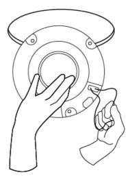
3. Make sure the mounting feet are turned inward to clear the opening and insert the speaker into the ceiling or wall. Position the speaker into the hole.
