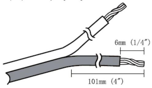
When you are ready to prepare your speaker wires, first separate about 4" of wire, then strip about 1/4" (6mm) insulation from the end and twist it to prevent stray strands. If you plan to use banana or pin plugs (highly recommended), install the plugs on the wire.
