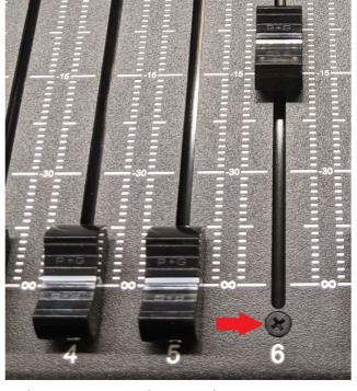
• STEP 3 Flip the unit over to access the fader port. Remove the two screws and remove the cover
