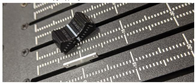
• STEP 2 Remove the screws that hold the fader in place. One above
