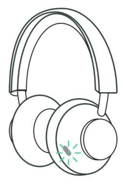
3. The green indicator flashes slowly (Ss/time), the Bluetooth pairing is successful: two Bluetooth playback devices can be used at the same time.
