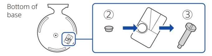
4. Attach the base, and then secure with a screw. Use a coin or similarly shaped object to tighten the screw.
