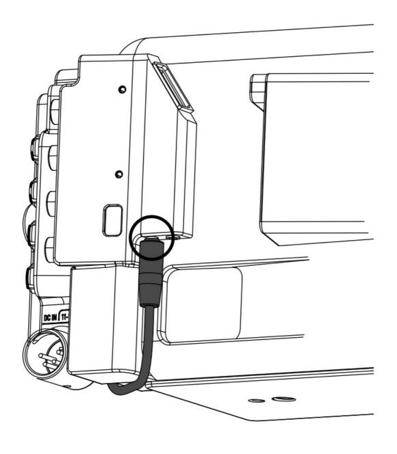
Attach to camera using V-Mount interface.
