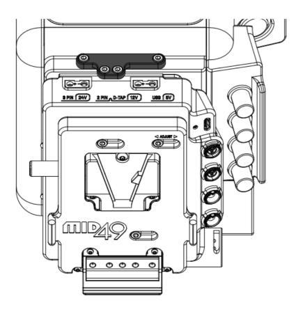
When using wide batteries, adjust battery plate position to expose power outputs.
