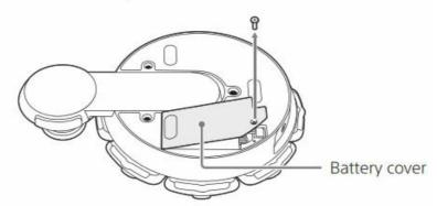
4 Detach the connector from the battery. Remove the battery.
