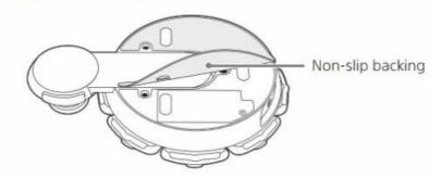
3 Use a crosshead screwdriver to remove the screw on the battery cover. Remove the cover.
