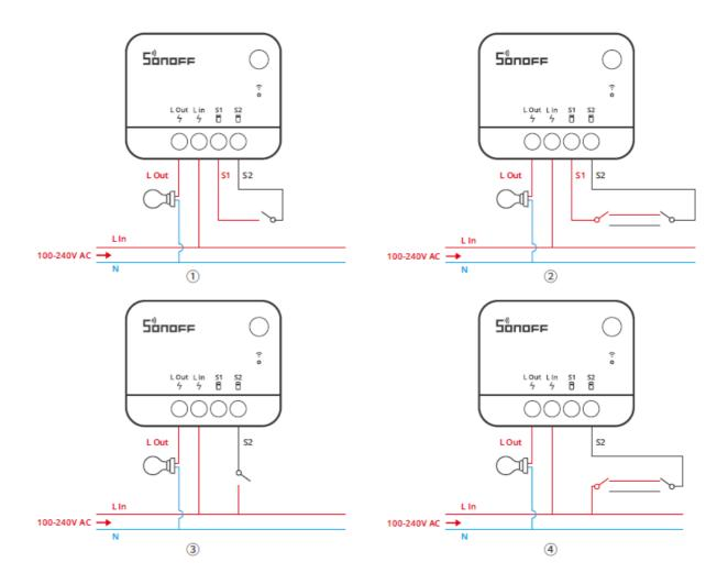
For the above 3.4 wiring methods, please ensure the proper wiring and powering of the L in the terminal, otherwise, it will cause the device to work abnormally.
